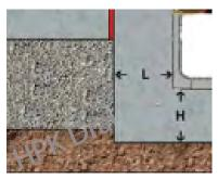
Asphalt - Load up to Class C
