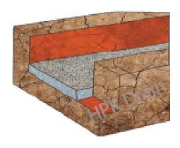
2: Concrete Base: lay the concrete base to the recommended thickness as specified in table 2.10 using a minimum strength of 20 MPA. Allow enough gradient in the base for water drainage.
