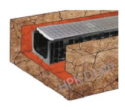
1: Excavation Design: the size of the trench will need to take into account the dimension and rating of the channel in determining the depth and width of the trench (See Table). The trench should be excavated from the lowest point of discharge to the highest point. The base should be compacted well particularly if the ground is soft.
