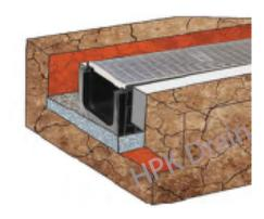
3: Channel Installation: assemble the channels including fixing the grates to the channels and position inside the trench starting from the lowest point of discharge ensuring that each channel unit is locked securely together and aligned. Place concrete along the sides of the channel making sure that it worked into the ribbing along the base as well as sides paying particular attention to the grate support edge.
