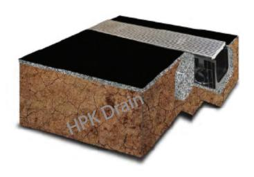
HPK drainage systems require the strengthening of concrete to support loads of vertical and horizontal thrust. In creating a concrete haunch to lock the channel, it enables it to meet the required load rating as specified in AS4058 - 2006.
